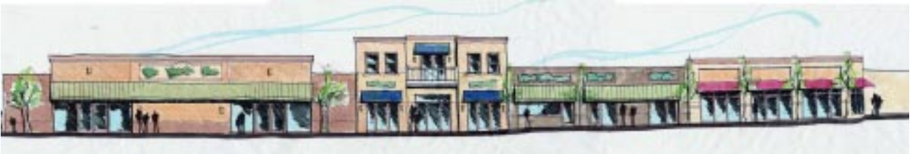
Elevation of proposed improvements illustrates how display windows, color, appropriate signage and varying the height of buildings can create a more dynamic retail image.
